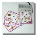
The chip card reader is required to transfer information from the PC onto the chip cards. For example if the cards are to be loaded by means of money software or to transfer vending information from the PC onto the coffee machine.
