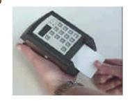
The hand held loading station is used to load money cards in remote locations. For example the switch board could have a unit to load staff cards. This will eliminate the need to go to the coffee machine in order to load the cards. It is powered by a 9 V battery, which makes its operation independent from power supply. A power adaptor is also available for 110 Volt operation.
