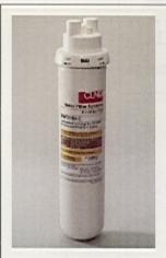
The CUNO® Series 6000 are complete single vessel systems designed for ease of operation and contain an automatic valve that stops the water flow simply by twisting the cartridge. This feature not only eliminates the need for external valves, but also prevents the water supply from being accidentally turned on with the cartridge removed. Systems are designed to remove hardness, sediment, taste and odor.
